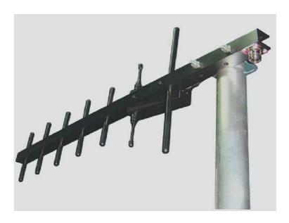
The antenna designed for a base installation, in telecommunication networks to increase the range of radio modems operating at the band of 868 MHz. A duraluminum construction is powder painting and DC-grounded makes it resistant to environmental conditions with a special consideration of mountain installations, hard-available high masts, maintenance-free systems, etc.
