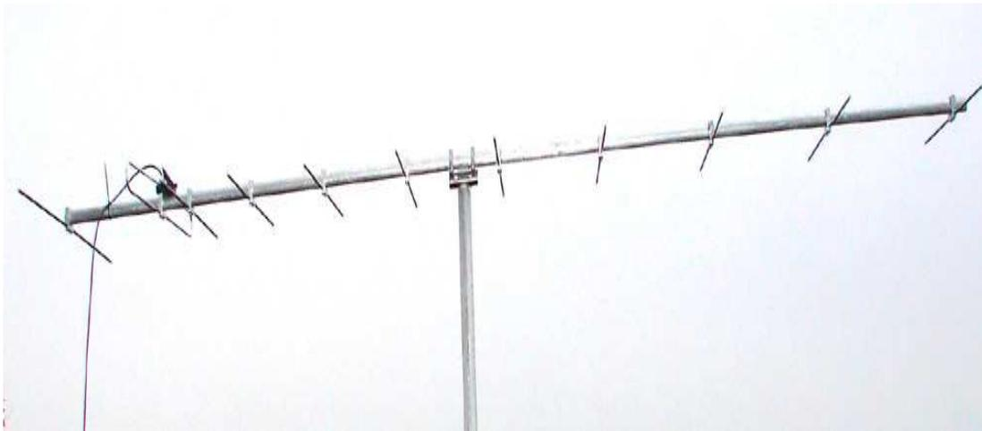
**A typical 11-element Yagi antenna matching with a loop. A duraluminium construction may be fold out to transport. All screw connections are made of stainless steel, a PA7 alloy ensures required stiffness. A practical mounting enables install at vertical and horizontal polarization. Dimensions of antenna were optimized with a special consideration of wide bandwidth and keeping a high gain. The antenna may be produced for another frequency from the range 140 – 460 MHz .**
